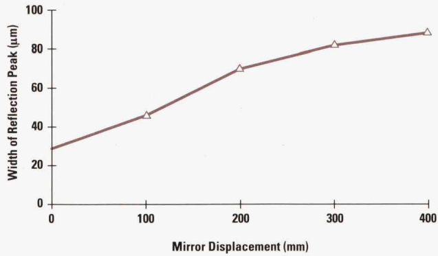
Fig. 7. Degradation of the spatial resolution in the HP 8504A precision reflectometer made with an LED source operating at 1550 nm.
